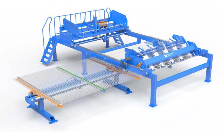
>The line wires are automatically arranged and pushed together and fed
